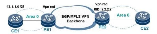
As shown in the figure, a CE requires access to the Internet, and PE 1 is connected to the Internet gateway. Configurations on PE 1 are as follows: PE 1: # nat address-group 0 175.31.1.3 175.31.1.10 # ip vpn-instance vrf1routedistinguisher 192.168.1.1:100
