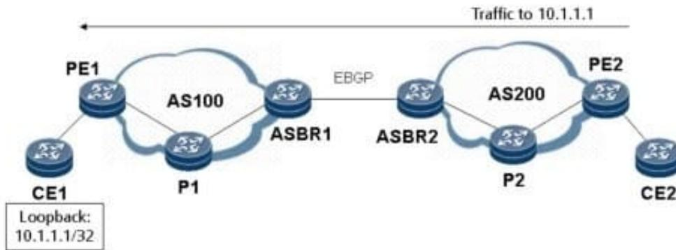
As shown in the figure, inter-AS VPN Option A is used. CE 1 and CE 2 belong to the same VPN. AS 100 and AS 200 run IGP and LDP, respectively. ASBRs communicate with each other through EBGP. The loopback interface address of CE 1 is 10.1.1.1/24. Suppose CE 2 can ping CE 1. Which router allocates an inner label when PE 2 forwards packets from CE 2 to CE 1?
