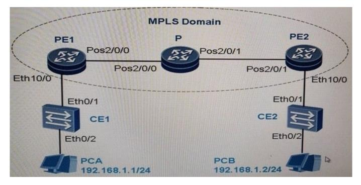
As shown in the figure, virtual private LAN service (VPLS) is enabled on routers PE 1 and PE 2.CEs are connected to PEs through QinQ and PC A and PC B are connected to the two CEs. The two PCs belong to the same VPN and can communicate with each other properly. Which of the following statements about the communication process when you ping PC B from PC A are true?
