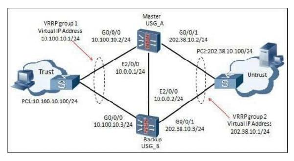
When USG\_A is in failed state, such as power failure, this time USG\_B state switched from Slave to
