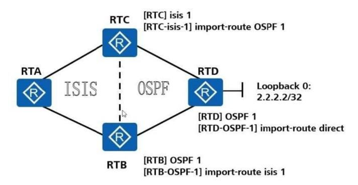
A. The following configuration can be performed on RTC to filter out only routes to the network segment 2.2.2.2/32 when RTC imports routes:[RTC] ip ip-prefix 10 index 1 deny 2.0.0.0 8 less-equal 32[RTCisis-1]filter-policy ip-prefix 10 import
