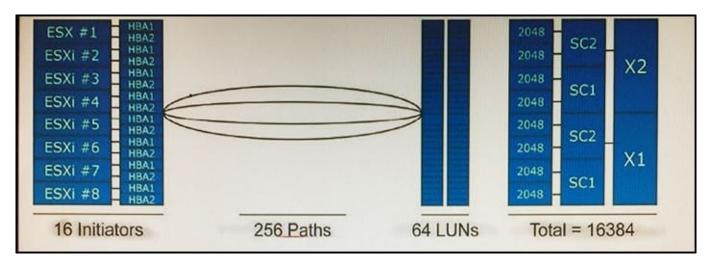
As shown in the exhibit, a customer\\'s environment is configured as follows: Dual X-Brick cluster 8 ESXi hosts with 2 HBAs Each ESXi hosts has 8 LUNs Each LUN is visible through 4 paths
