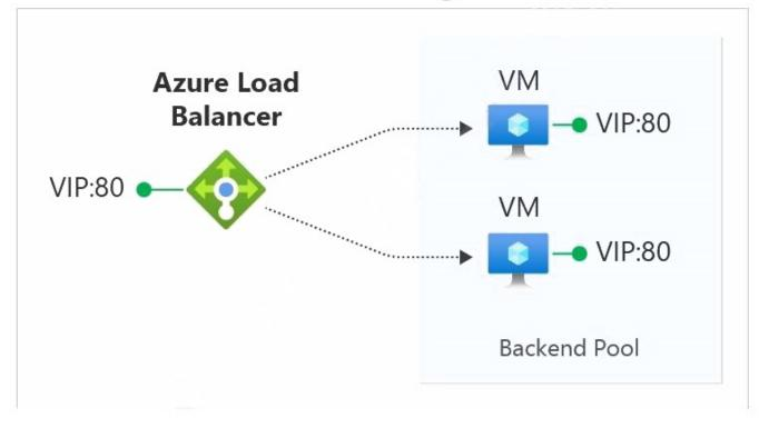
Load-balancing rules - A load balancer rule is used to define how incoming traffic is distributed to the all the instances within the backend pool. A load-balancing rule maps a given frontend IP configuration and port to multiple backend IP addresses and ports.
