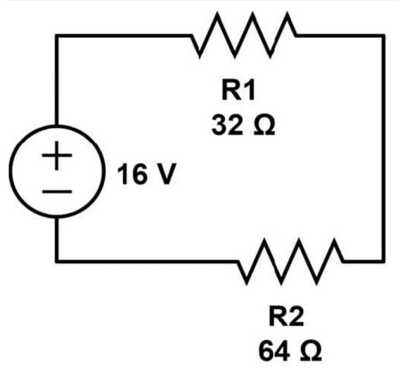
Given the electrical circuit in the image provided, what is the current in resistor R1?
