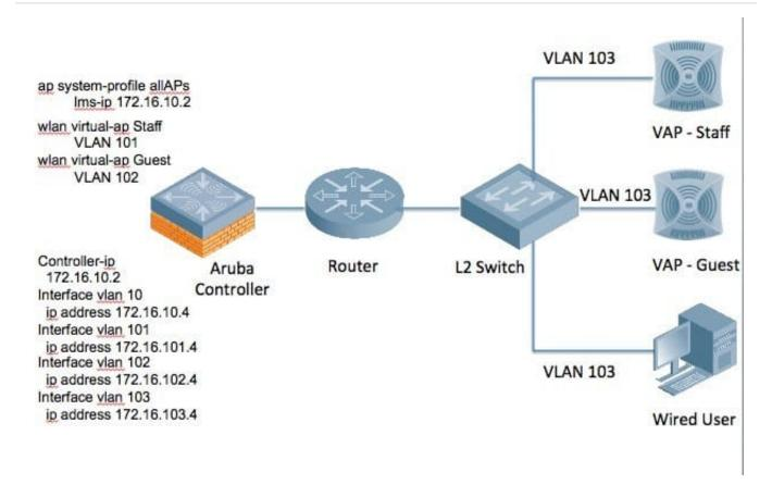
Which VLANs must be configured on trunk link D between the router and Aruba controller to support wireless users when the controller is provisioned for L2 operations?
