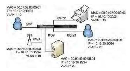
Referring to the exhibit, which interfaces will receive a packet sent to MAC address 00:05:85:7F:EB. 80 from the user with IP address 10.10.10.10?
