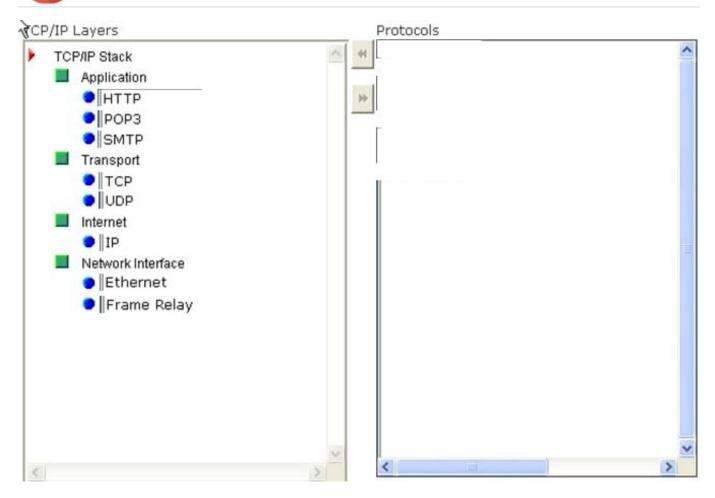
TCP/IP defines a large set of protocols that allow communication between various devices on a network. TCP/IP classifies the various protocols into different layers. Some of the common protocols are listed in the table below:
