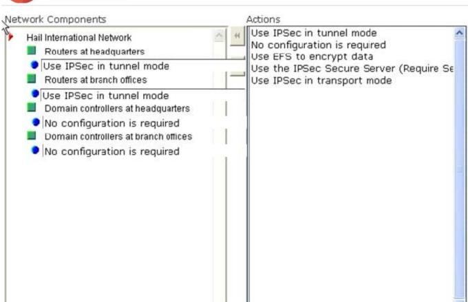
In order to accomplish the task, you will have to configure the routers at all locations to use IPSec in tunnel mode. Tunnel mode protects the WAN traffic. If you configure IPSec on routers, no security for the WAN communication is required on other servers and workstations.
