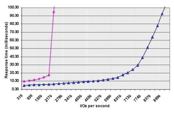
An administrator is checking the load on the array. The administrator is trying to determine if this is an acceptable range (between 8370 and 8990 IOPs). Based on the illustration, what can you conclude?
