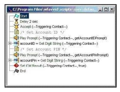
A. The "Set Contact Info" variable should be used before the "Set ICM Result" to set "Call.PeripheralVariable1". to "accountID" and "Call.PeripheralVariable2" to "accountPIN"
