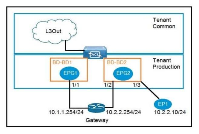
Refer to the exhibit. An engineer wants to avoid connectivity problems for the endpoint EP1 when it reaches an external L3Out network through the gateway 10.2.2.254/24. Which two configurations must be implemented in BD-BD2? (Choose two.)
