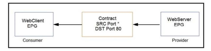
Refer to the exhibit. Which combination of flags in the Cisco ACI contract allows a client in WebClient EPG to establish an HTTP connection toward a server in WebServer EPG?
