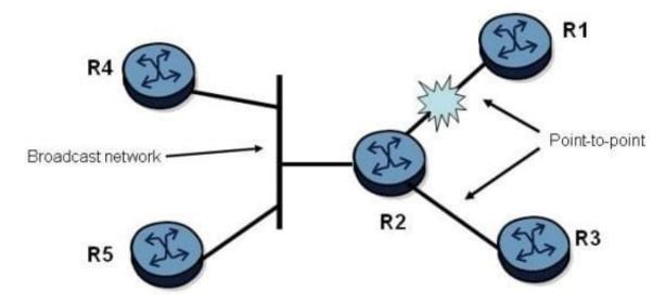
OSPF router R2 has both point-to-point and broadcast interfaces and it is not a DR for any interfaces. Router R2 detects the link failure between itself and router R1.
