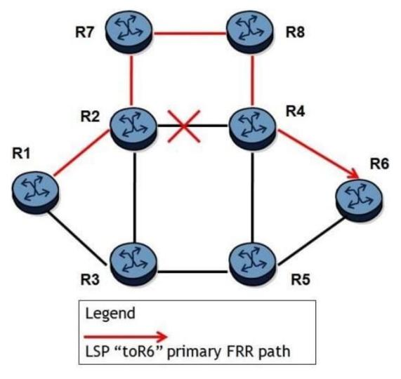
A fully loose LSP "toR6" is enabled with FRR protection. All links have the same cost. After the link between R2 and R4 goes down, FRR protection repairs the LSP and traffic traverses on R1-R2-R7-R8-R4R6. Which of the following about this CSPF-enabled LSP on an Alcatel-Lucent 7750 SR is TRUE?
