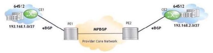
The AS-path nullification method is used to prevent CE2 from discarding routes received from CE1. On which router should the AS-path nullification policy be configured?
