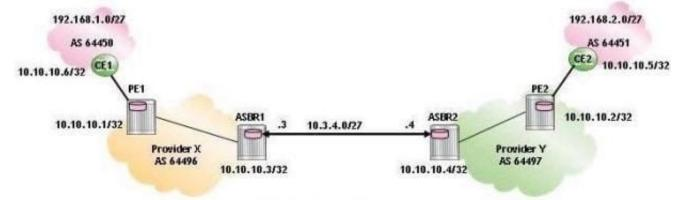
\*A:ASBR1>config>service>vprn# info description "Customer A" router-id 10.10.10.3 autonomous-system 64496 route-distinguisher 64496:1 auto-bind 1dp vrf-target target:64496:10 interface "toASBP2" create address 10.3.4.3/27 sap 1/1/2 create exit exit bap group "toASBR2" neighbor 10.3.4.4 export "mbgp-bgp" peer-as 64497 exit exit exit no shutdown
