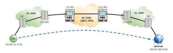
A Carrier Supporting Carrier (CSC) VPRN is configured for a customer carrier who is an Internet Service Provider (ISP). If CE1 sends an IP packet to 192.60.100.1, which of the following is FALSE?
