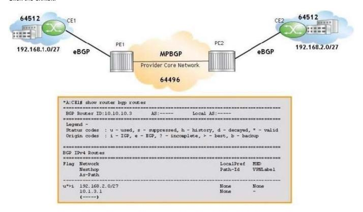
The CLI command "remove-private" is configured on PE1 to eliminate BGP loops in the VPRN. For the displayed route, what is the value of the AS-Path field?
