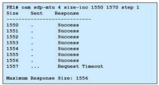
E-pipe 100 is using an SDP with an LSP that uses the path shown (PE1-PE2-PE3-PE4). Based on the OAM command output, which of the following is FALSE?
