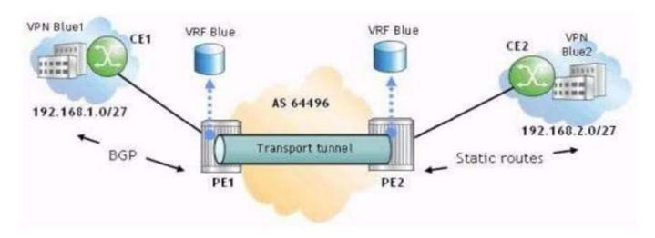
Routes are exchanged between CE1 and PE1 using BGP. CE2 and PE2 use static routes to forward traffic to and from the VPRN. Which of the following is FALSE?
