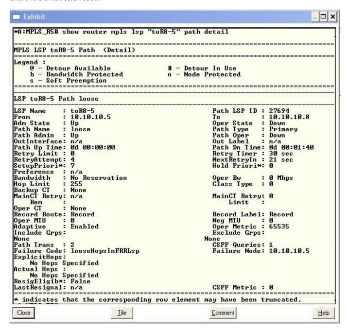
LSP "toR8-5" requests fast reroute protection on the primary loose path. What could be done to remove the Failure Code shown?
