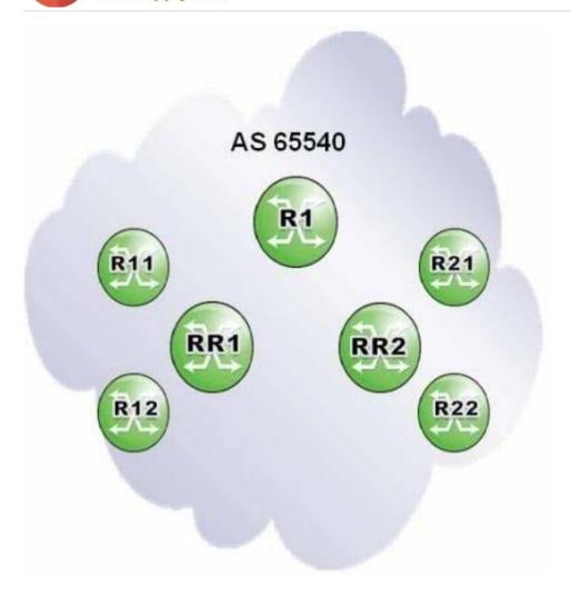
Routers RR1 and RR2are route reflectors with clients R1x and R2x, respectively. Routers RR1 and RR2 are non-clients of each other, and router R1 is a non-client of both.
