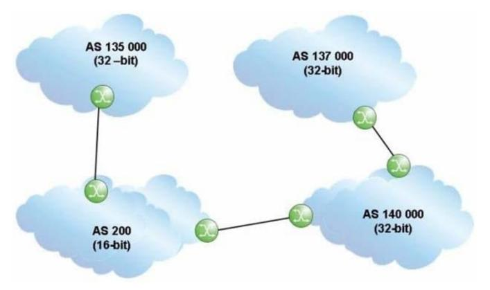
An update travels from AS 137000 to AS 135000, traversing both 32-bit and 16-bit AS Paths. What AS Path is seen by AS 200?
