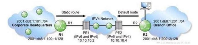
A service provider is deploying a 6over4 tunnel to connect a customer\\'s branch office IPv6 network to the corporate headquarters as shown in the exhibit. Which command is used to create a default route on PE2 for the branch office network?
