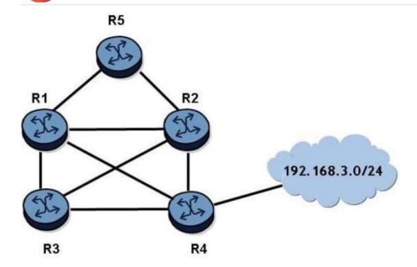
OSPF is operational on all links in the network diagram, all links have the same cost and all routers are configured with an ECMP value of 4. Router R4 advertises the prefix 192.168.3.0/24 into OSPF.
