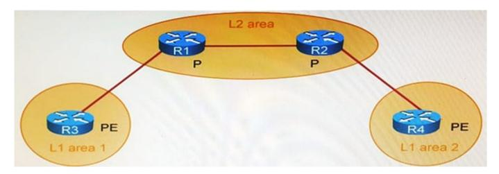
A. to build an LSP between the PE routers
