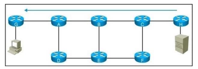
This network is running IS-IS as the single routing protocol and the LSP and SPF timers are aggressively configured so the network converges in subsecond. The customer reports that router B had a memory crash and reloaded, which resulted in some packets from the application being lost. The application servers are behind router G and the end users are behind router H. Which design change should be made to prevent this packet-loss problem from reoccurring?
