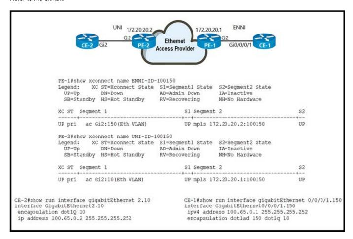
An Ethernet access provider is configuring routers PE-1 and PE-2 to provide E-Access EVPL service between UNI and ENNI. ENNI service multiplexing is based on 802.1ad tag 150, and service-multiplexed UNI is based on 802.1q tag 10. Which EFP configurations must the provider implement on PE-1 and PE-2 to establish end-to-end connectivity between CE-1 and CE-2?
