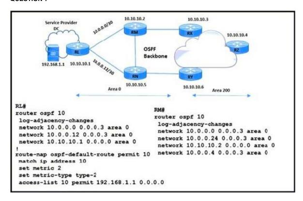
Refer to the exhibit. The operations team for a service provider network is implementing a route map policy. OSPF area 0 should originate the default route with a type 2 metric of 2 when the application server on the connected interface
