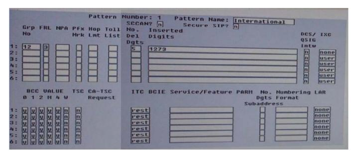
Consider the settings shown in exhibit displayed by using the display route ?pattern command. You must deny calls from users in COR 10 to use route pattern 1. What should the fault restriction level (FRL) for COR 10 be?
