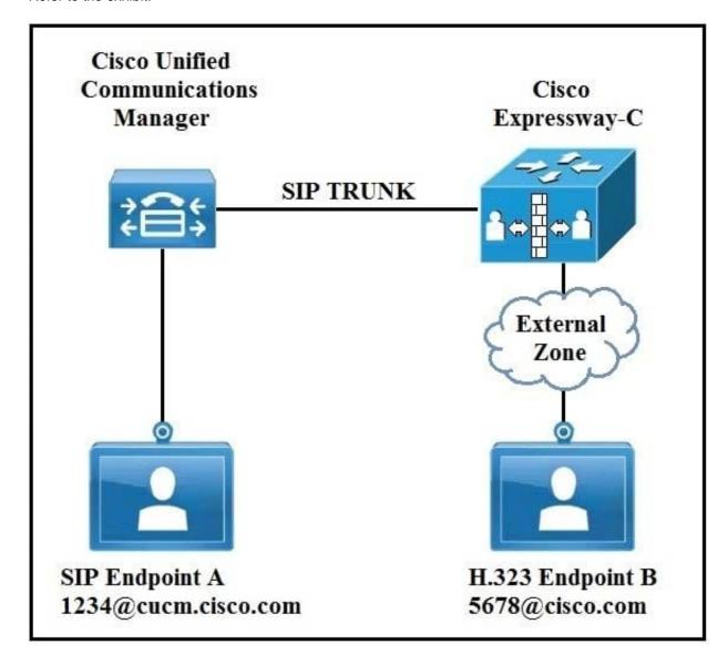
In an environment SIP devices are registered to CUCM and H.323 devices to VCS. What would be required to enable these calls to setup correctly?
