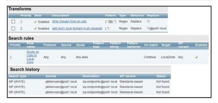
Calls to locally registered endpoints are failing. At present, there are two endpoints registered locally to this Expressway. An H.323 endpoint with an alias of "EndpointA" is registered, and a SIP endpoint with an alias of "EndpointB@pod1.local" is also registered.
