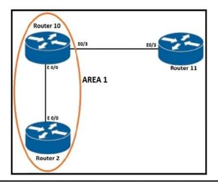
R10#debug condition interface ethernet0/0 Condition 1 set R10# debug ip ospf packet OSPF packet debugging is on \*Feb 19 01:43:27.659: OSPF-1 PAK : Et0/0: IN: 10.2.10.2->224.0.0.5: ver:2 type:1 len:44 rid:10.0.0.2 area:0.0.0.1 chksum:E41B auth:1 \*Feb 19 01:43:29.035: OSPF-1 PAK : Et0/0: OUT: 10.2.10.10->10.2.10.2: ver:2 type:1 len:44 rid:10.0.0.10 area:0.0.0.1 chksum:CE86 auth:1
