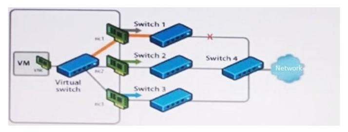
Each ESXi host has three NICs assigned to a virtual switch.
