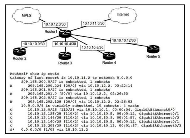
Which next-hop IP address does Router1 use for packets destined to host 10.10.13.158?
