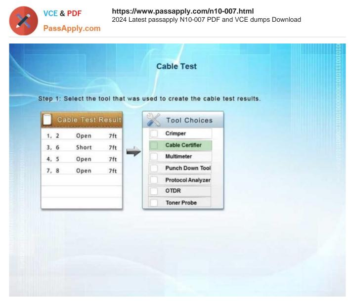
A Cable Certifier provides "Pass" or "Fail" information in accordance with industry standards but can also show detailed information when a "Fail" occurs. This includes shorts, the wire pairs involved and the distance to the short. When a short is identified, at the full length of the cable it means the cable has not been crimped correctly.
