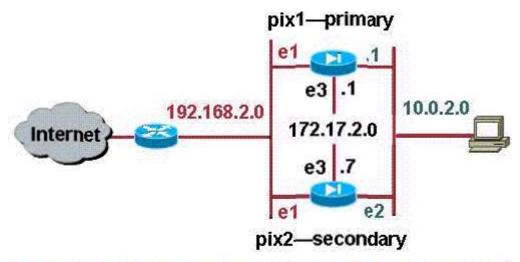
pix2(config)# failover lan interface LANFAIL ethernet3 pix2(config)# failover lan unit secondary pix2(config)# failover lan key 1234567 pix2(config)# failover lan enable pix2(config)# failover
