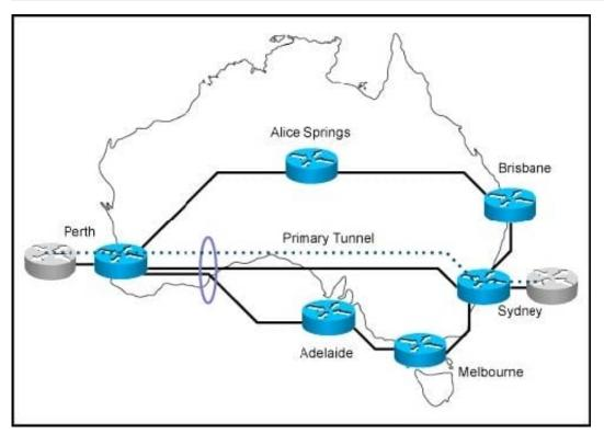
You are designing MPLS-TE for this network. The links form Perth to Sydney and from Perth to Adelaide share the same optical fiber in one given segment. Which feature should you implement to eliminate the risk that a backup tunnel is installed over the same optical fiber as the primary one?
